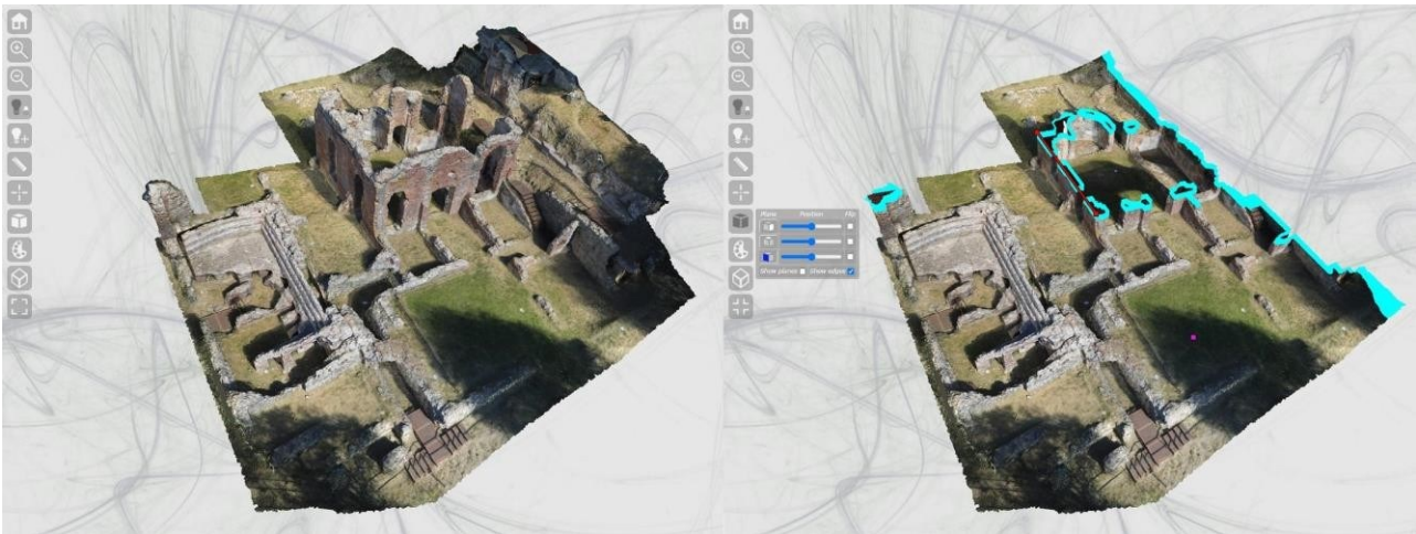
Fig. 4. The 3D model as displayed in 3DHOP. On the right, some of the features provided by the program: coordinate (purple) and distance (red) calculation, and cross-sections (cyan) (© MAPPALAB-UniPI).
